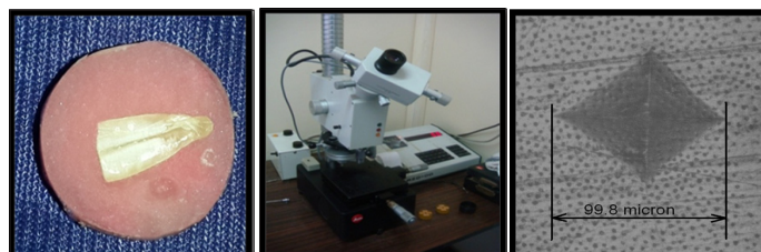
[Table/Fig-2]: Prepared samples; [Table/Fig-3]: Vicker's micro hardness tester machine; [Table/Fig-4]: Indentation marked in the mid-root region.
